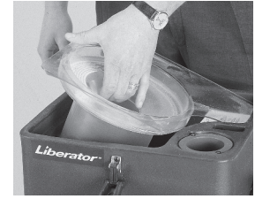
Remove the separator assembly to clean the vacuum cone.
